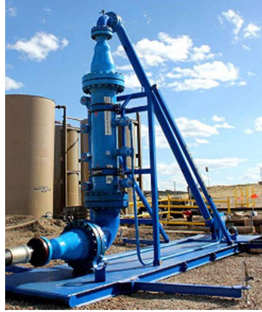
FIG. 4. (Color online) The AOT device is placed downstream next to the pump.
