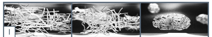
Figure 1: Molecular simulation of a solution of microcrystalline waxes in a hydrocarbon under a high strength electric field over time.
